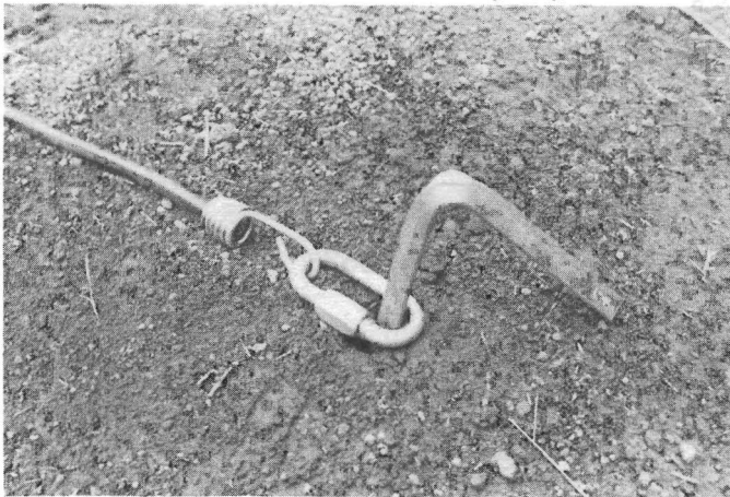
Figure 2.—Anchor stake and dragline attachment for portable rocket-nets.
